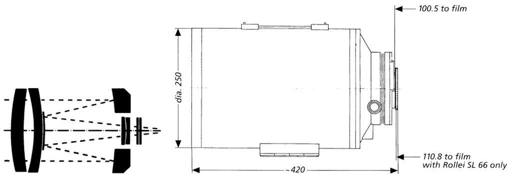
The basic design of the **Mirotar<sup>®</sup>** lens - concave primary mirror with a hole in the center and convex secondary mirror - is similar to the design frequently applied in astronomical telescopes. It further contains two lens elements in front of and two behind the mirror surfaces. They reduce the aberrations caused by the mirror to a minimum.
