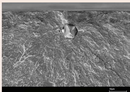
Scanning electron microscopic image of a 5µm oxide inclusion as a failure initiating site. The component failed due to a fatigue crack which was originated at the top of the unwanted feature in the microstructure within the (535A99) 100Cr6 matrix.
